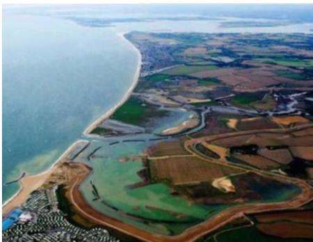
The Reserve was created in 2014 following construction, by the Environment Agency, of 4.25 miles of new floodbank inland from the sea between Selsey and Bracklesham. The existing shingle beach was then breached to create the largest managed realignment scheme on the open coast in Europe, creating amazing new wetland habitats surrounded by wide walking and cycling pathways. [See further information about the RSPB Reserve.](#)
